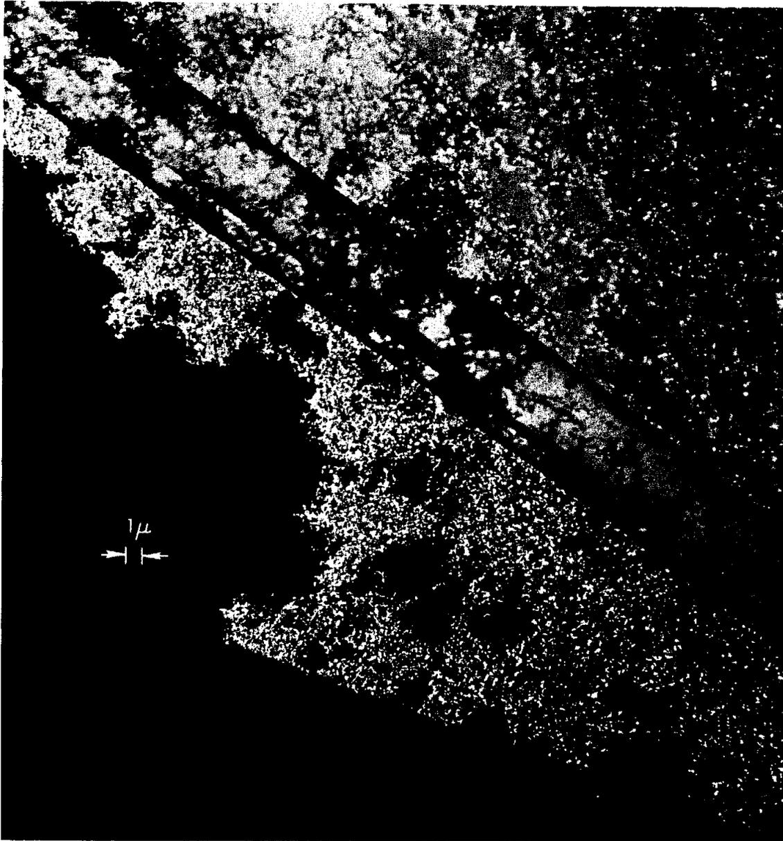
FIG.21-- CROSS SECTION OF A LOW DENSITY KCl DYNODE TAKEN ON AN ELECTRON MICROSCOPE AT 4,000 X.
