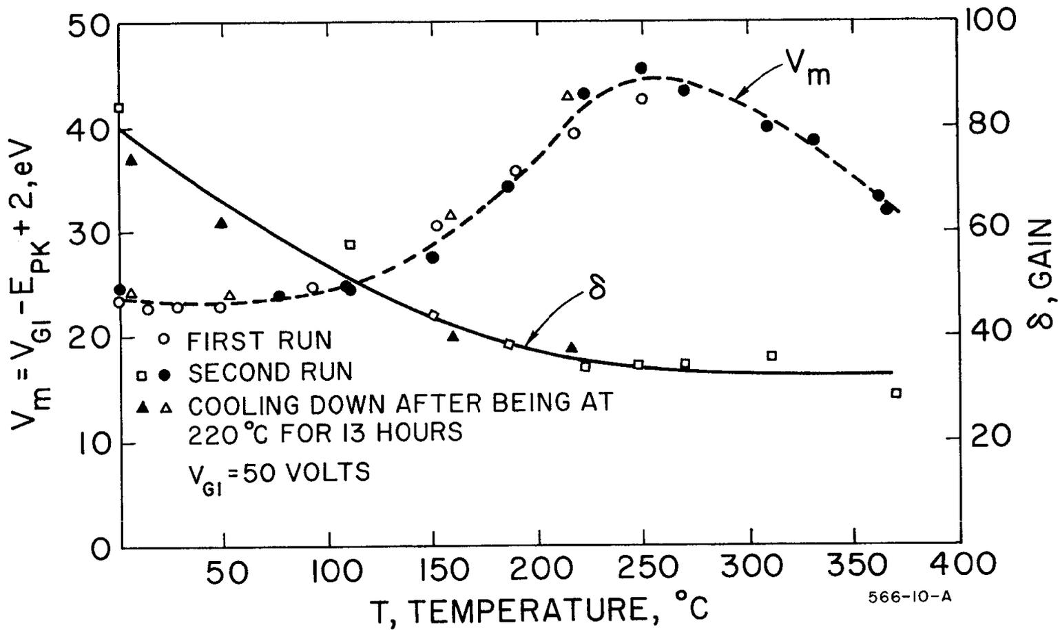
Fig. 20 - LIMITING EXIT SURFACE POTENTIAL ( $V_m$ ) AND GAIN ( $\delta$ ) AS A FUNCTION OF TEMPERATURE FOR A LOW DENSITY KCl DYNODE
