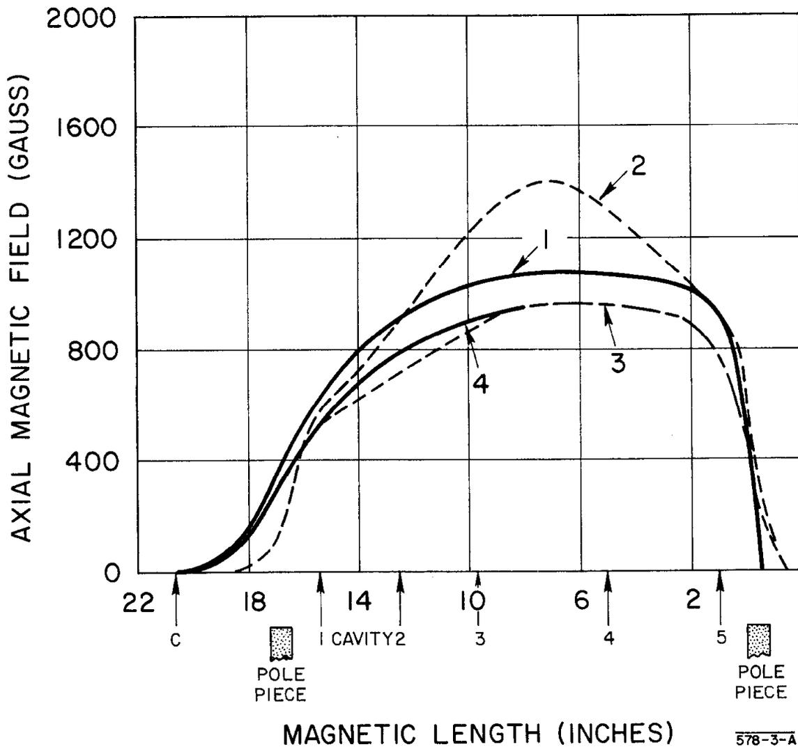
FIG.10--AXIAL MAGNETIC FIELDS FOR STANFORD KLYSTRONS
