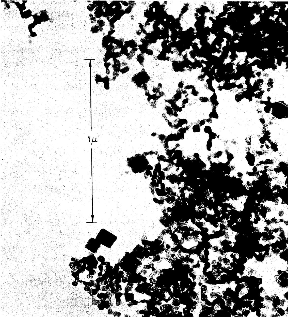
FIG. 22 -- CROSS SECTION OF A LOW DENSITY KCl DYNODE TAKEN ON AN ELECTRON MICROSCOPE AT 100,000 X.
