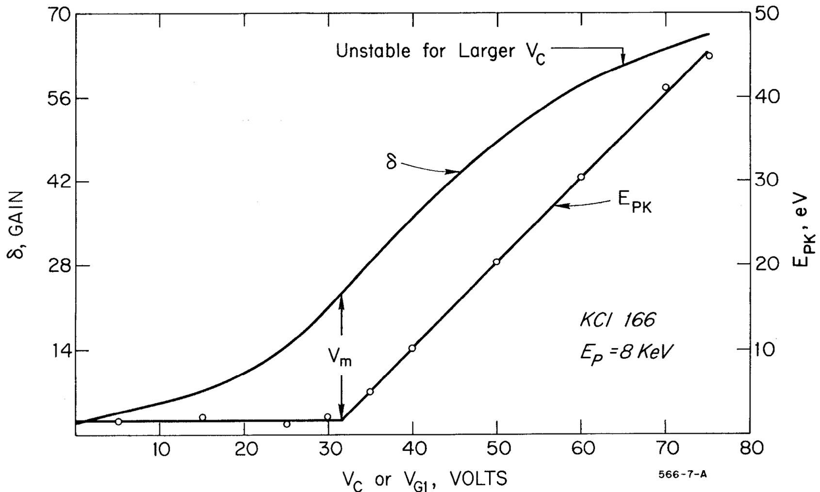
Fig.19-ILLUSTRATING THE LOCATION OF  $V_m$  ON THE  $\delta$ vs  $V_C$  CHARACTERISTIC FOR THE LOW DENSITY DYNODES
