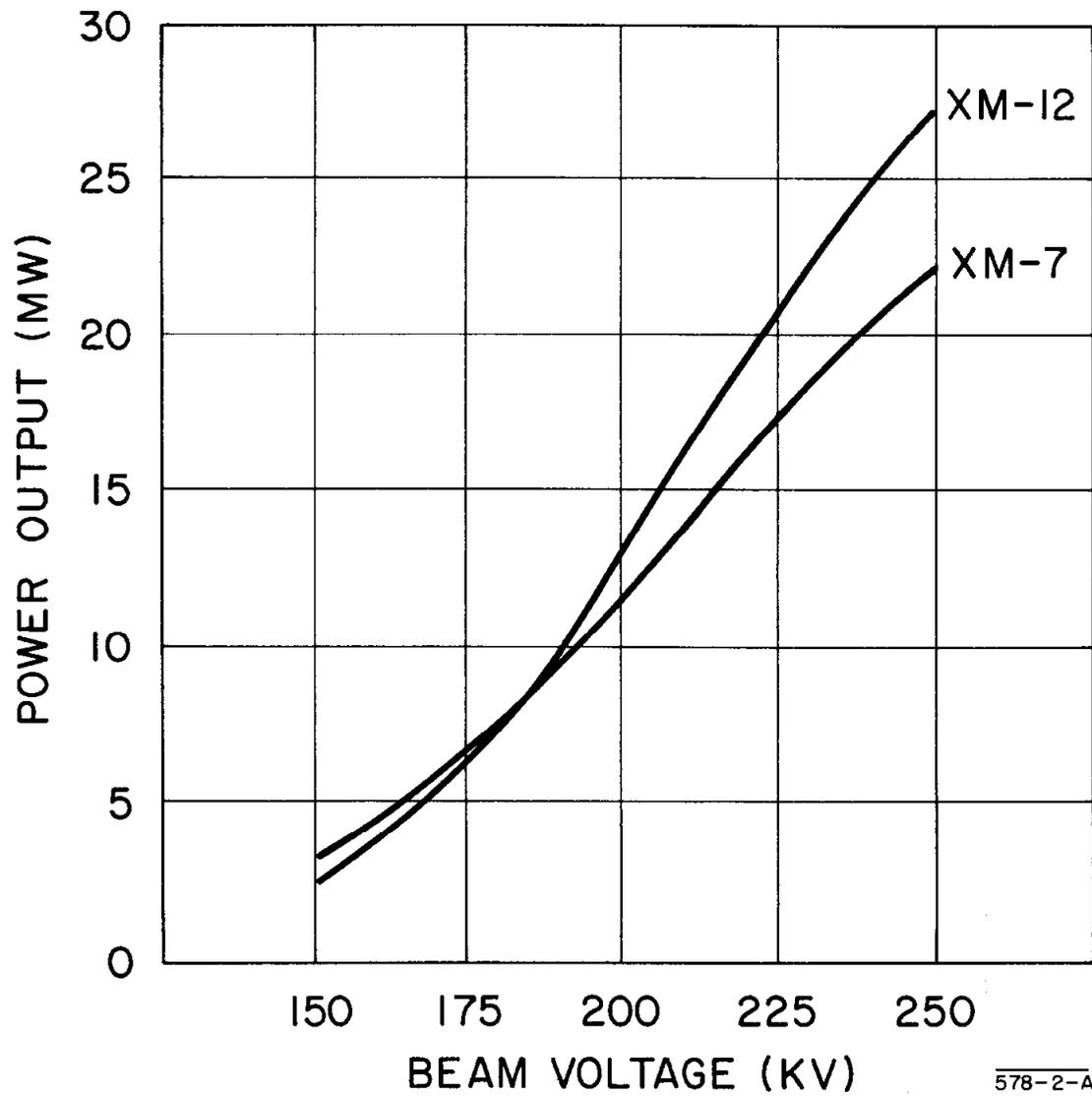
FIG. 11 -- STANFORD KLYSTRON PERFORMANCE
