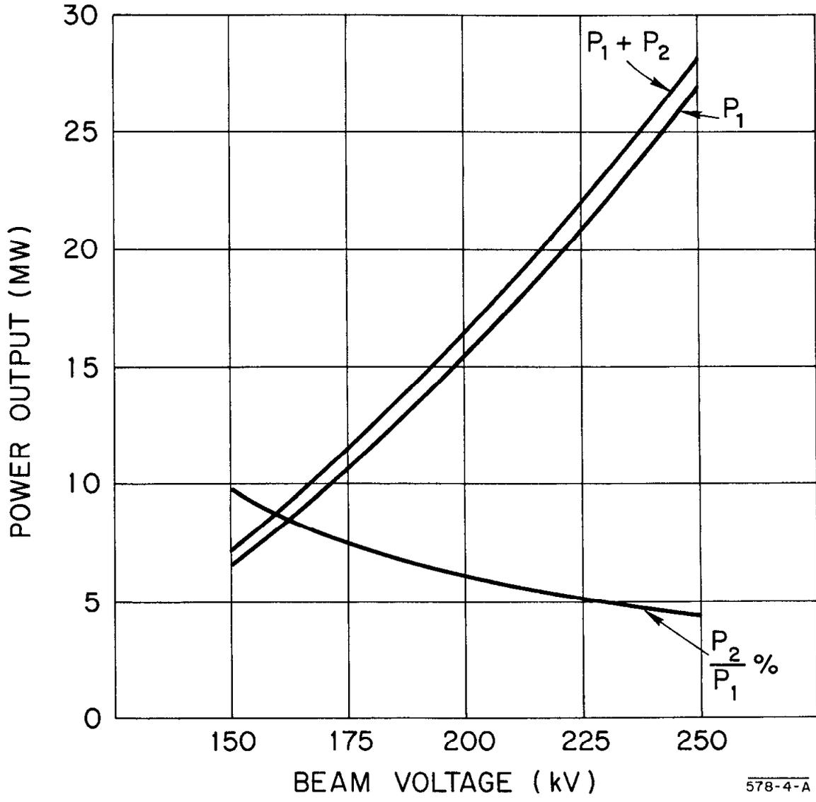
FIG. 9 -- EXPERIMENTAL DOUBLE OUTPUT KLYSTRON PERFORMANCE
