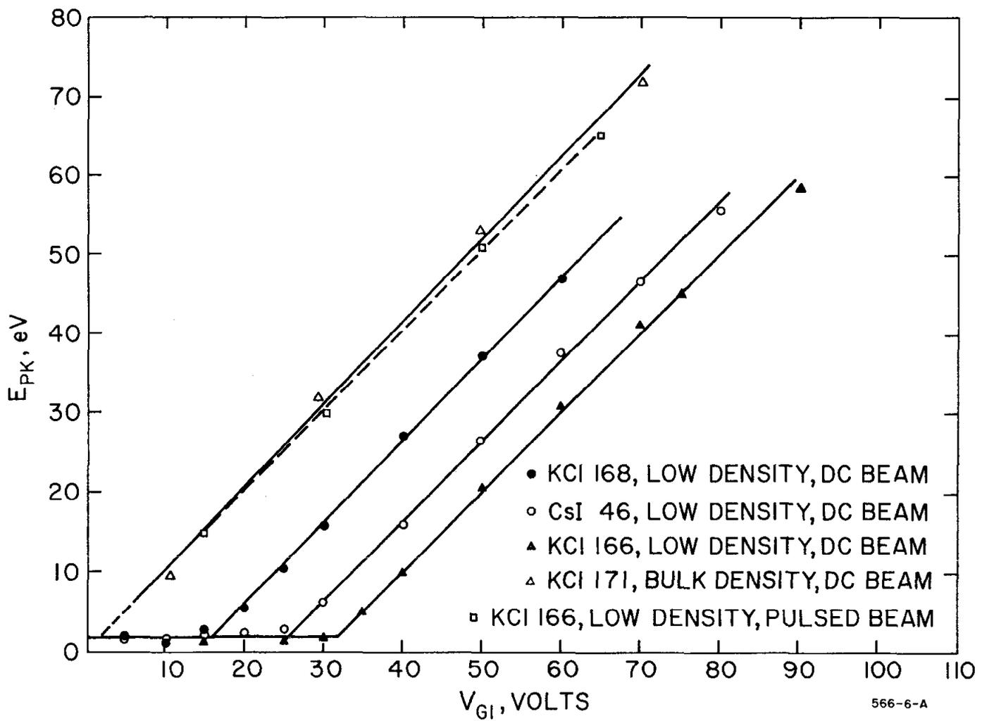
Fig.18-MOST PROBABLE SECONDARY ELECTRON ENERGY,  $E_{PK}$  (measured at  $G_1$ ) vs. THE FIRST GRID POTENTIAL FOR LOW DENSITY AND BULK DENSITY DYNODES
