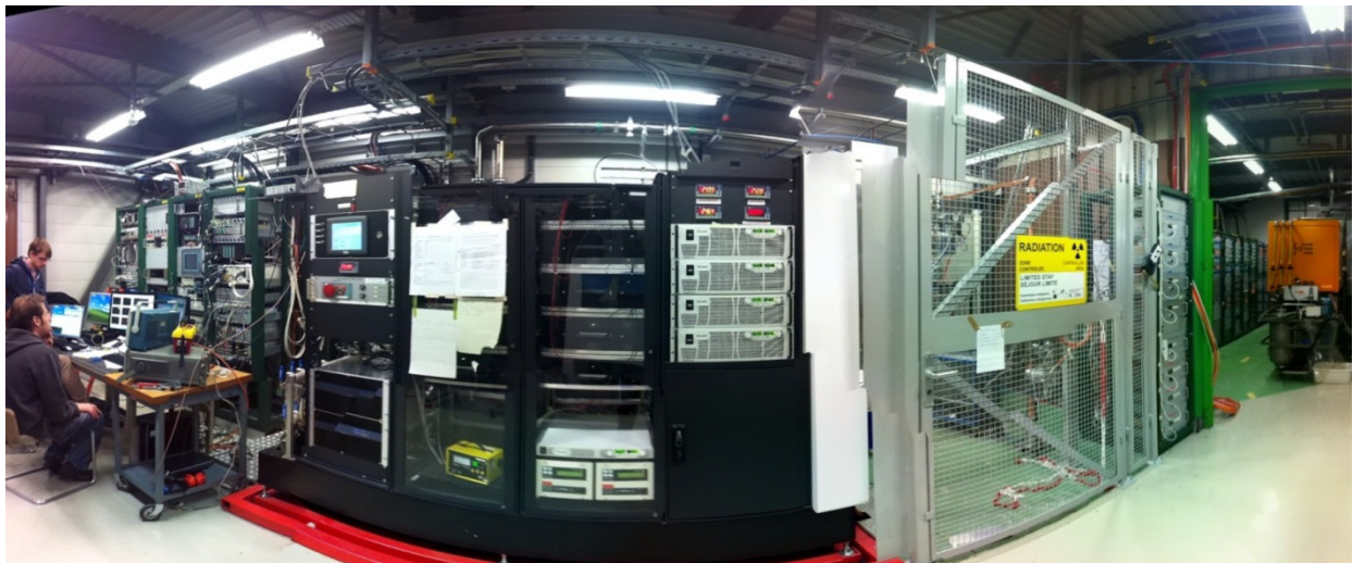
Figure 1: A photograph of the Xbox-1 test stand. The control and low-level rf systems are to the left, the modulator is in the middle and the high-power rf network is to the right. The test accelerating structure is located in the former CTF2 accelerator bunker located in the floor below.
