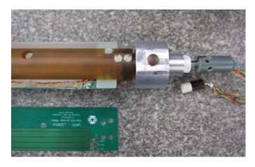
Fig. 5. Strong-back support of PCB probe which allows for different width circuit boards to be tested.
