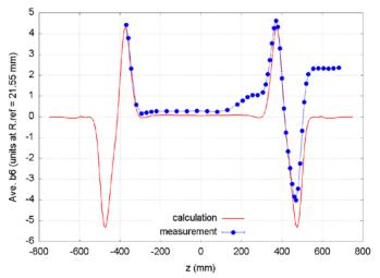
Fig. 7. 100mm long, 47mm diameter PCB measurement (DQB winding) of HQ01d quadrupole with calculation (note that the calculation did not account for the ramp splice region whose effect is seen on the measured data between 150-300mm on the z scale).
