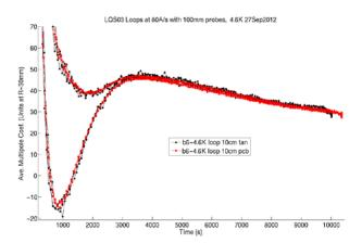
Fig. 9. PCB and tangential probe  $b_6$  comparison, LQS03
