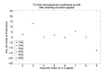
Fig. 10. Ferret measurements at various rotation rates in a superconducting Tevatron dipole.
