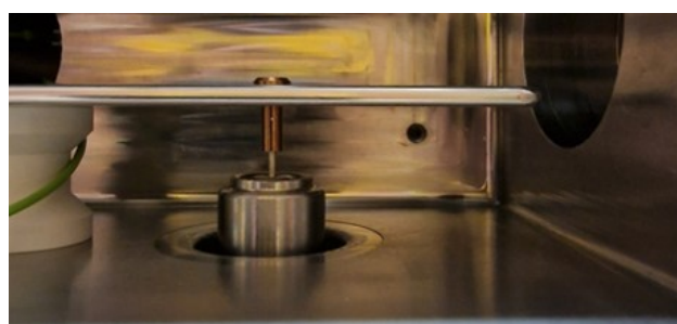
Figure 7: Feedthrough to electrode test assembly.
