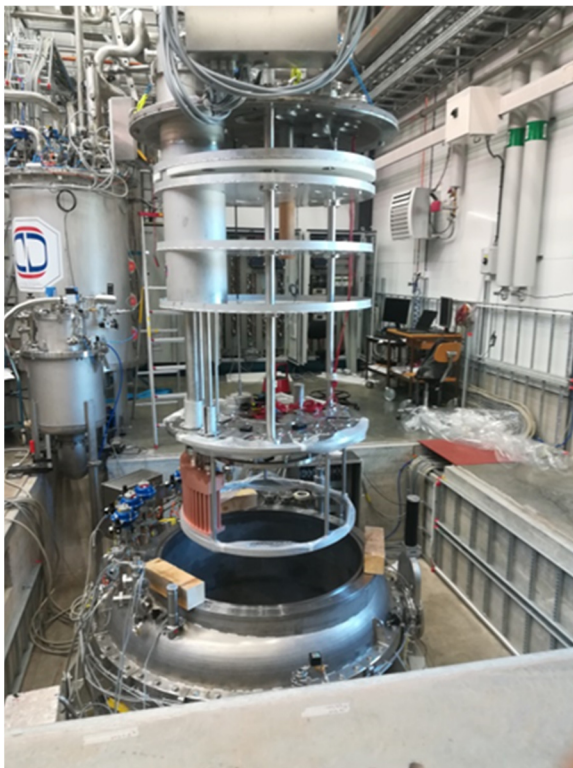
Figure 2: The GERSEMI Vertical cryostat and the magnet insert.
