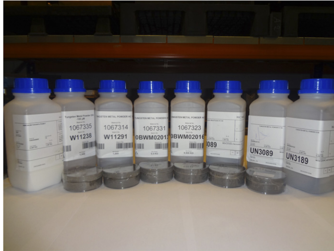
Figure 2. Assembly of all W powders provided by HCS Hermsdorf for HPGe \gamma -ray spectroscopic measurements.
