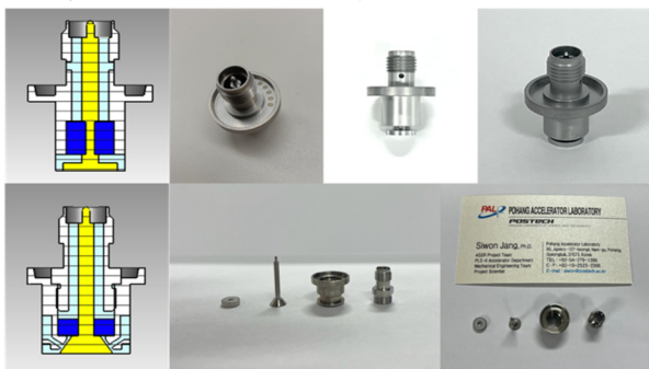
Figure 3: The final designs of the two types of antennas completed through optimization, as well as the prototypes of the antennas. The \text{SiO}_2 antenna is shown at the top, and the \text{Al}_2\text{O}_3 antenna is shown at the bottom.
