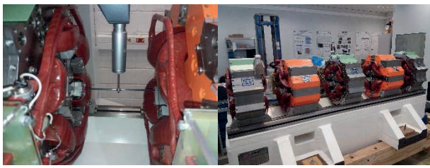
Figure 4: Girder set measured by a CMM (left) and by a laser tracker (right).
