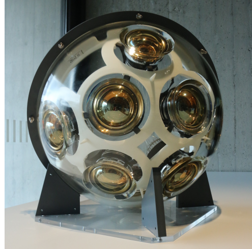
Figure 3: Picture of a mechanical prototype of the P-OM, with 8 PMTs optically coupled to the glass via gel pads.
