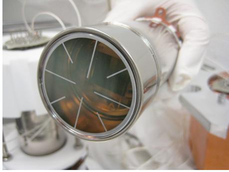
Figure 3.19: Picture of the R8778 PMT used by the LUX experiment. The PMTs are cylindrical, with 5 cm diameter. Photo courtesy of C. Hernandez Faham.
