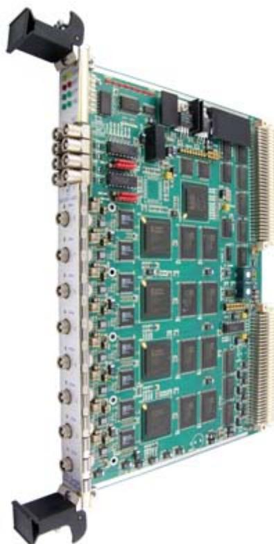
Figure 3.6: Picture of the Struck SIS3301 Fast ADC module used in the XENON10 data acquisition system. The modules feature 105 MHz digitization rate, and 14-bit resolution with a 2V dynamic range.
