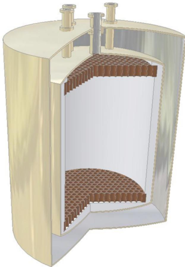
Figure 8.6: Baseline design of the LZ20 detector, with a 20 T active liquid Xe mass.
