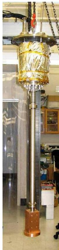
(b) Picture of the LUX power thermosyphon, showing the Cu head at the bottom, which connects the detector to the thermosyphons and delivers  $> 1$  kW cooling power.
