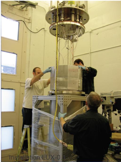
(a) Al displacer block (250 kg) being installed inside the LUX0.1 detector
