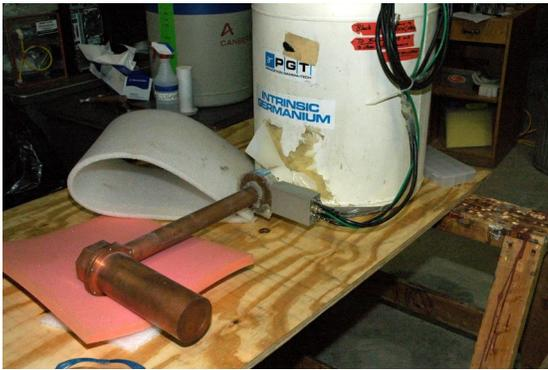
(a) Diode-M detector, outside of shield
