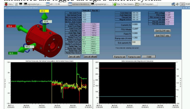
Figure 3: Solenoid control GUI, developed using EPICS EDM.
