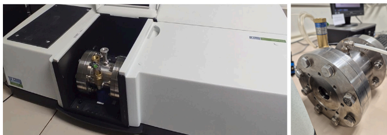
Fig. 2. Setup for the measurement (and monitoring during ePIC dRICH operation) of the C 2 F 6 transparency in the 200–900 nm wavelength range.
