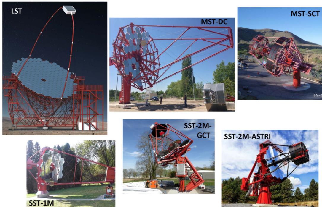
Figure 3.20: In this figure, from Ong [82], we can see all six of the candidate telescope designs 5 .
