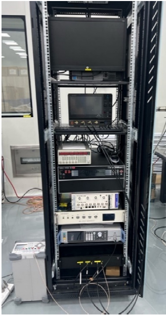
Figure 3: A 19" electronic rack with the depth 800 mm for BSM test bench electronics housing.
