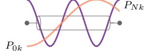
Figure 8.10: The sign of \mathbf{P}_{0k}\mathbf{P}_{Nk} indicates if ends of the chain oscillate in phase, or in phase opposition, in the mode k .
