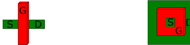
Figure 1.10: Conceptual diagram of a linear transistor (left) and an enclosed layout transistor (ELT) (right))
