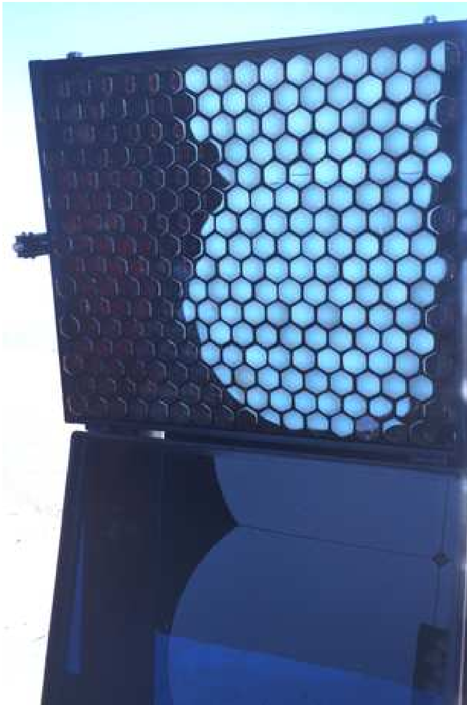
Figure 3.2. A HiRes2 cluster box with the UV filter lowered. The cluster contains 256 photomultiplier tubes arranged in a tightly packed hexagonal array of 16 rows and 16 columns. On the left the YAG laser fiber for this mirror can be seen. Half of the mirror is seen reflected on the cluster box.
