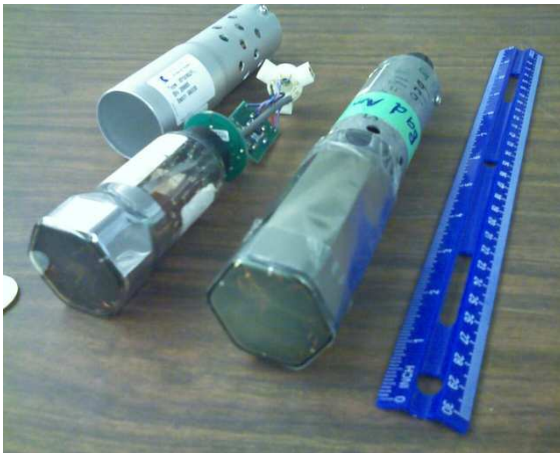
Figure 3.15. A HiRes photomultiplier tube. Each tube views about 1^\circ cone of the sky. The disassembled tube on the left shows the small circuit board that contains the preamplifiers. The hexagonal shape of the tube face can be clearly seen here.
