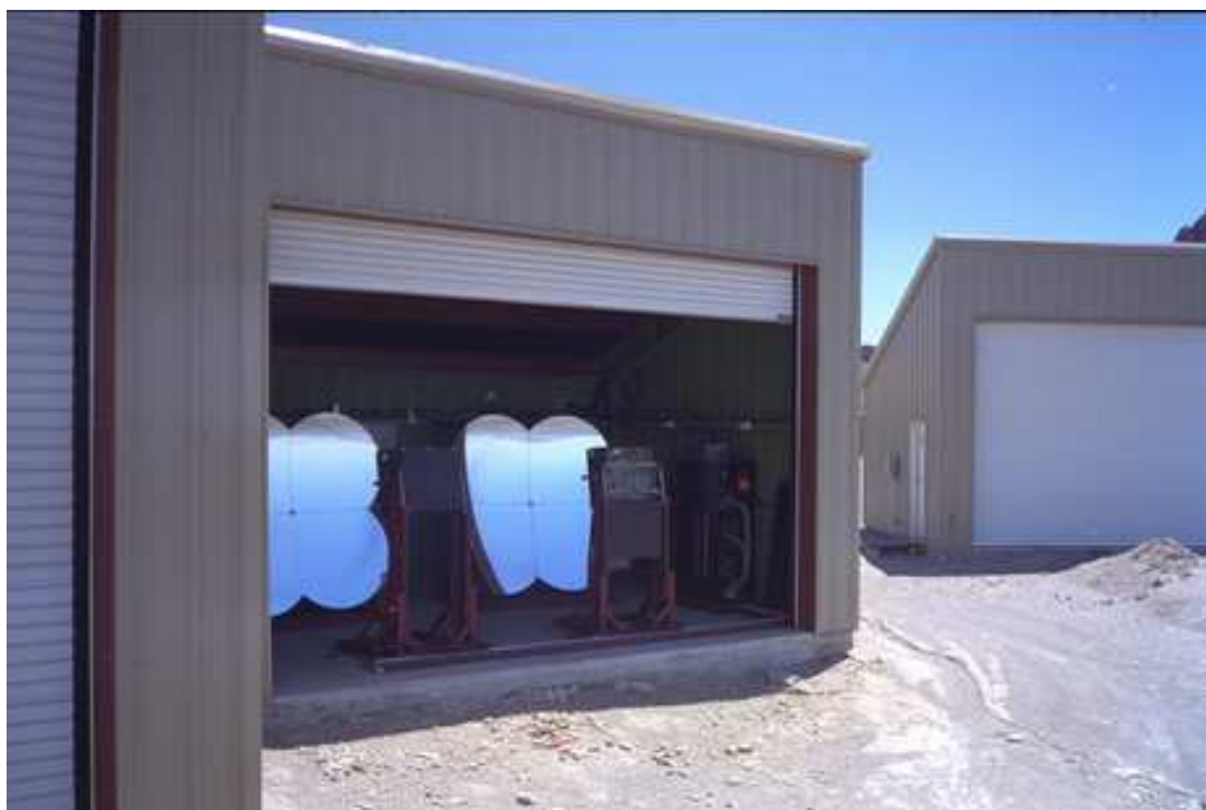
Figure 3.1. Two mirrors at HiRes2. The segmented cloverleaf construction is clearly visible here. In front of each mirror is a photomultiplier tube cluster box. The electronics rack which controls both mirrors is visible to the right of the mirrors. The protective door is raised here and can be seen in the lowered state on the building to the right. These are ring 1 mirrors that view from 3^\circ to 17^\circ in elevation.
