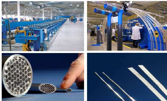
Figure 16: View of the production hall (upper left and right) and the HTS wire at different steps of the manufacturing process (lower left) and the finished HTS wire. Picture from AMSC.
