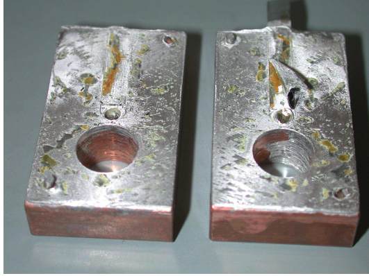
Figure 60: Reopened copper block, the non uniform surface hints that the soldering was only partly successful.
