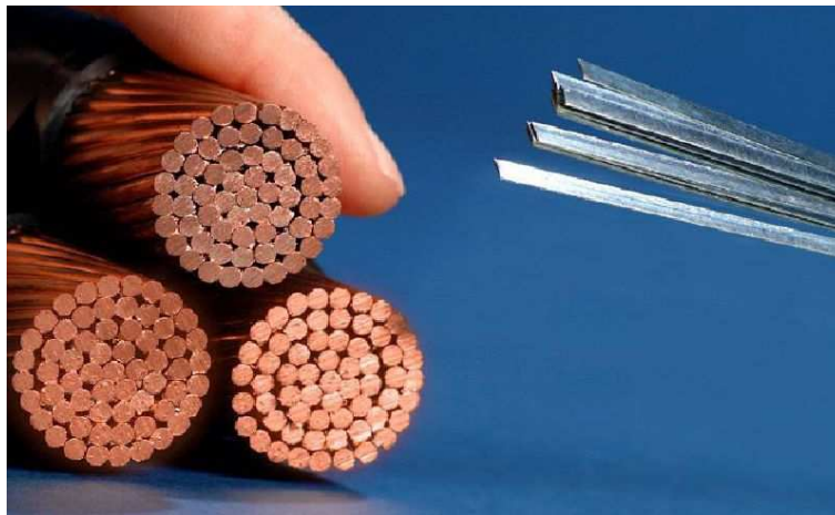
Figure 15: Comparison of the cross section of a normal conducting wire and a HTS wire carrying the same current (low temperature, no external field). Picture from AMSC.
