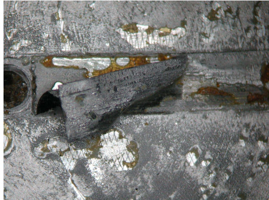
Figure 61: Expanded view of the copper block surface, remains of the flux and not soldered areas are visible.
