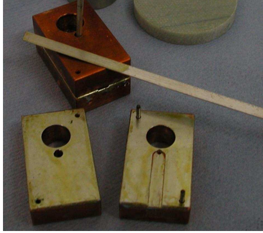
Figure 44: Two halves of a copper connection showing the groove and the soldered surface.
