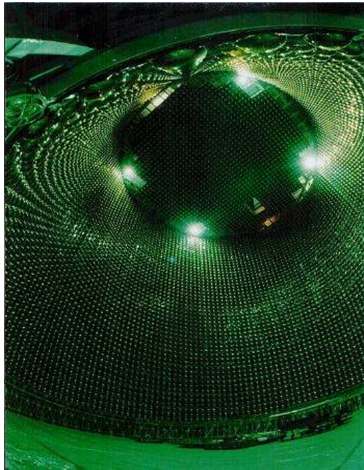
Figure 3: The SUPERKAMIOKANDE detector, wall and top with about 9000 photomultiplier tubes which are used to measure the Cherenkov light of crossing neutrinos. Picture from the SUPERKAMIOKANDE collaboration web site.
