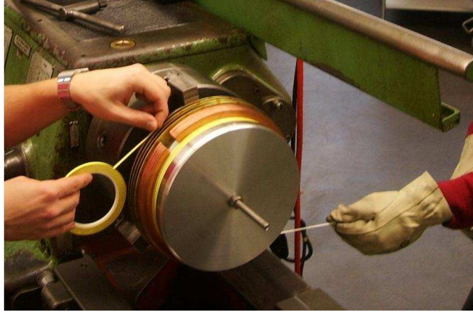
Figure 84: Picture of the winding process on a lathe. The HTS wire coming from the right is insulated with the yellow tape.
