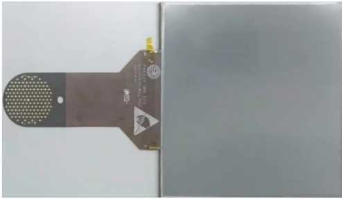
Figure 2. One Micromegas module produced by USTC. A mesh layer is bonded on a Kapton based flexible printed circuit board (PCB), with pillars in between creating a 100\ \mu\text{m} gap. A layer of germanium is coated on the PCB surface to quench sparks.
