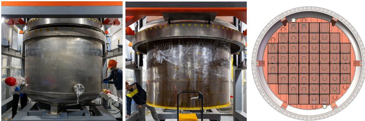
Figure 1. (Left): The PandaX-III detector vessel. (Middle): The field shaping cage mounted on the top flange of the detector. It is made of flexible PCBs and a acrylic barrel. (Right): The preliminary design of the readout plane on top of the field cage, which holds 52 Micromegas modules in total.
