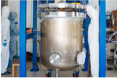
Figure 4. The vessel of the PandaX-III prototype detector with an inner volume of 600 L. It accommodates 7 Micromegas modules inside.
