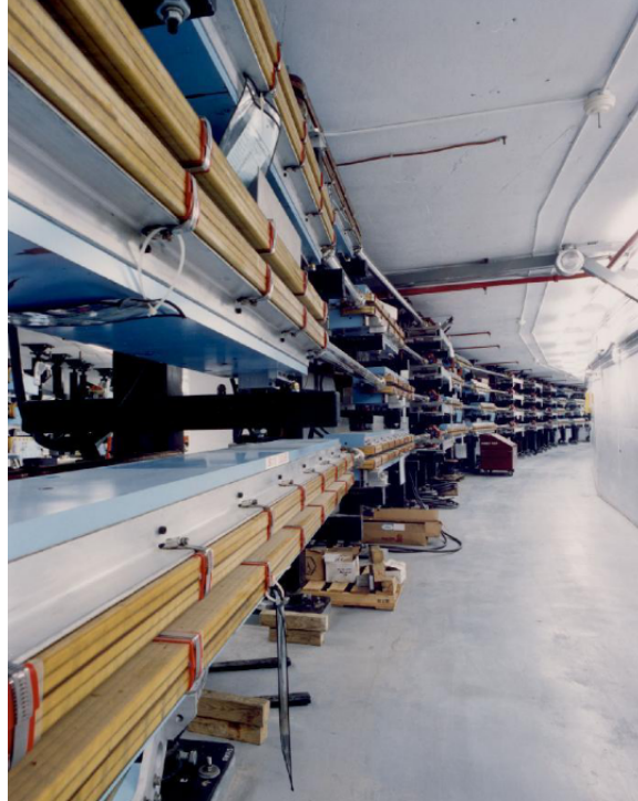
Figure 17: A picture of recirculation arcs [79] utilizing dipole magnets to bend electron beam by 180^\circ .
