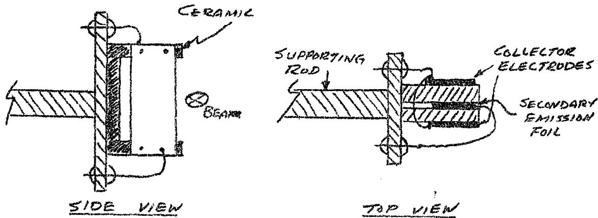
SUPPORTING ROD TO BE CONNECTED TO ADJUSTABLE BELLows —
