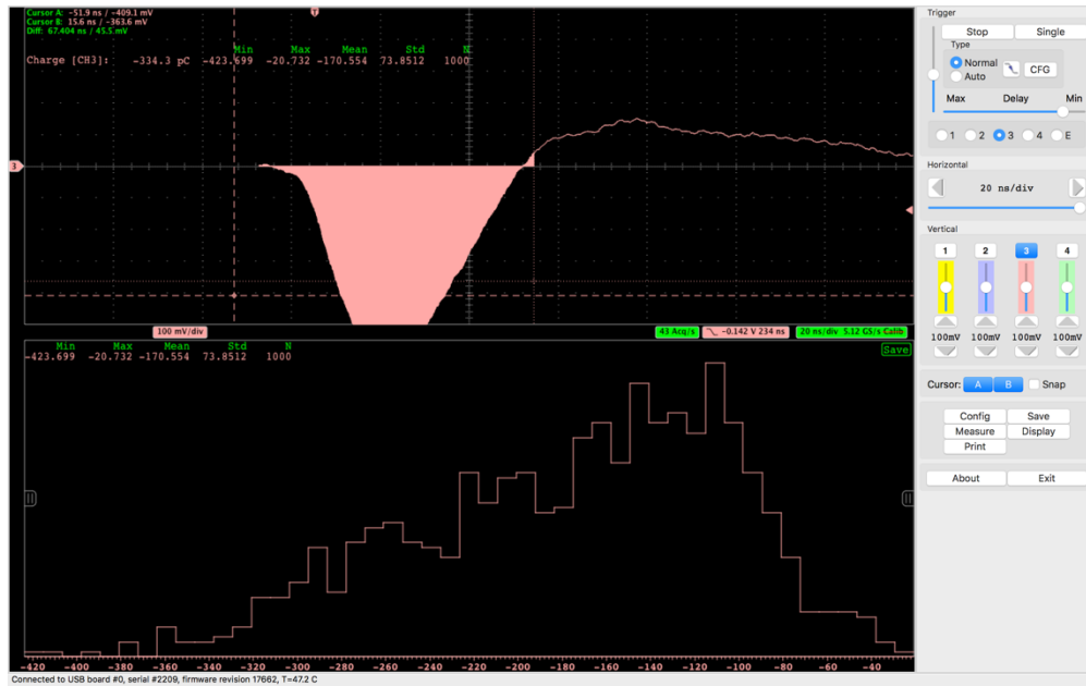
Figure 4.11: By adding optical grease it can be seen the signal amplitude increases to the peak value of 500mv, and the acquisition rate is also increased two fold.
