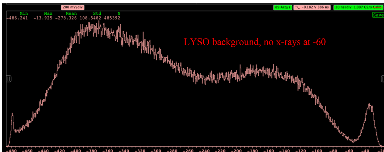
Figure 4.6: Characteristic background noise can be seen above. This noise comes from intrinsic background radiation found in LYSO crystals. We note that in the background noise a clear trend is found, in that no signal is detected at -60. This is ideal for the experimental setup, as the characteristic signal of radioactive Co is found at a value of -60. To insure this effect was due to intrinsic radiation of the LYSO crystal, the detector was placed in a lead pig for 2 hours to create the background noise seen above.
