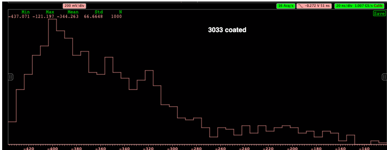
Figure 4.12: As can be seen above, a coated LYSO crystal has in general, a higher characteristic background energy. This allows the crystal to be useful in detection, as the background noise is nowhere near the characteristic signal detection of -60.
