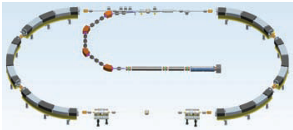
Figure 1: The layout of the iRCMS. The racetrack design consists of two 10.5 m long straight sections and two 180 degrees arcs of radius 5 m.
