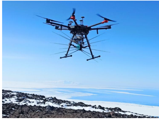
Figure 2: Drone-borne cal-pulser during the calibration of TAROG-M system in Antarctica
