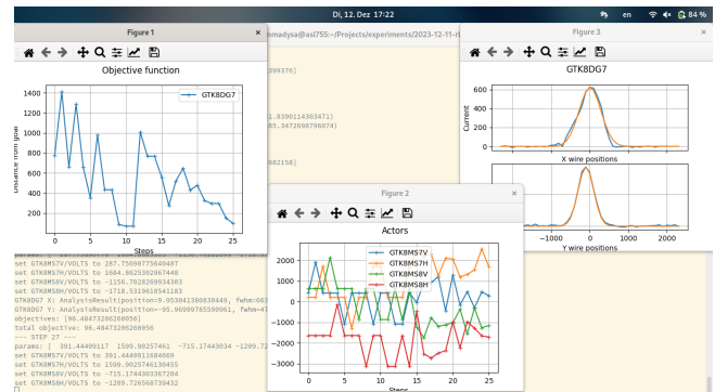
Figure 2: Screenshot of a typical optimization run using Geoff . Shown is the usage in a scripting context: the terminal window with logging messages is in the background, live graphs for monitoring in the foreground.
