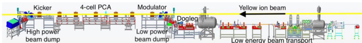
Figure 2: PCA-based CeC system installed at RHIC. The electron beam is generated in a 1.25 MV superconducting radio frequency (SRF) photo-electron gun, accelerated to 14.56 million electronvolts (MeV), and merged to co-propagate with the 26.5 GeV/u ion beam circulating in RHIC's yellow ring.
