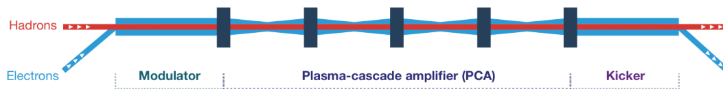
Figure 1: Schematic of a CeC system with the PCA at BNL's RHIC.
