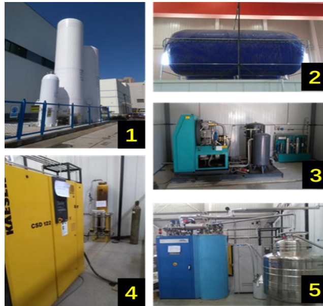
Figure 3. Cryogenic test station High pressure helium storage tank(1),Air bag(2), Compressor(3),TCF10(4), Liquid helium dewar(5).
