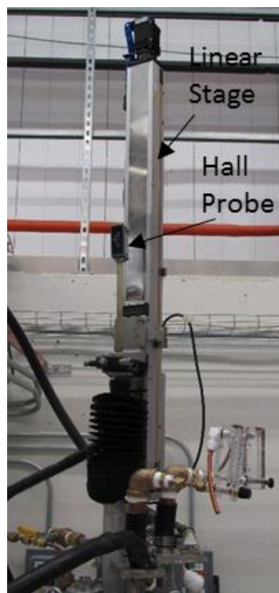
Figure 2. A photo of linear stage showing the hall probe tube connected to the stage, ready for scan.
