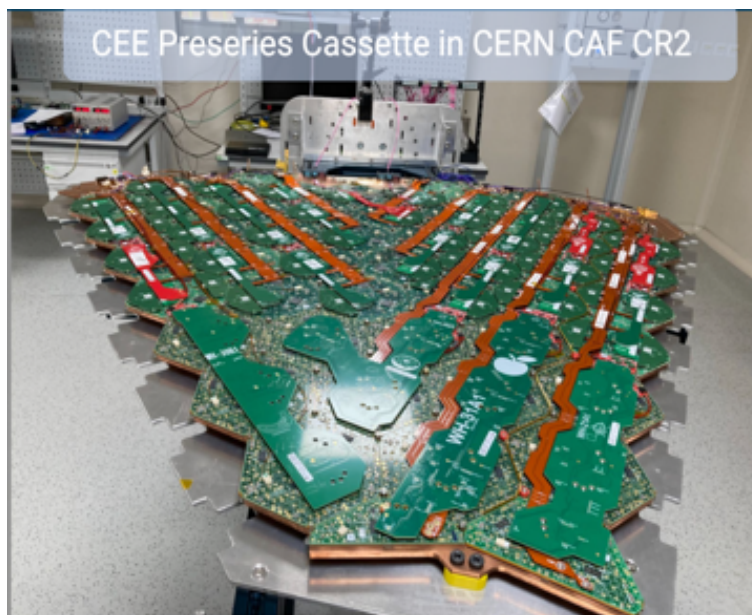
Figure 7. The HGCAL pre-series cassette assembled at CERN.
