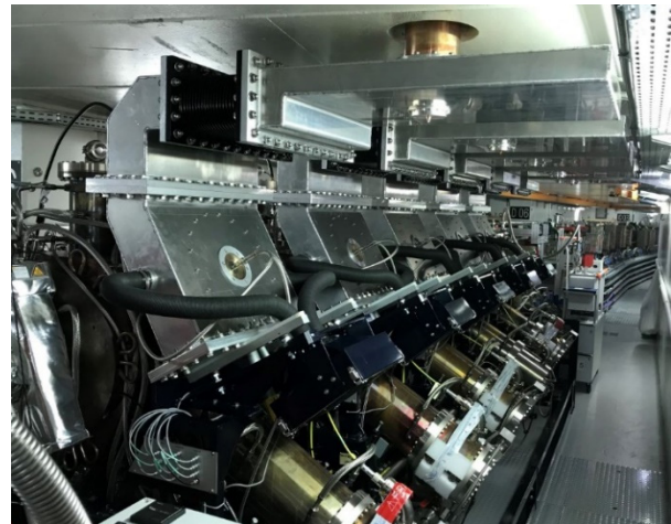
Figure 1: String of five HOM damped 352.37 MHz cavities in the EBS storage ring. Per cavity: R/Q = 145 \Omega , Q_0 = 35700 , R_s = 5 M\Omega , V_{acc-nom} = 500 kV, V_{acc-max} = 750 kV. Longitudinal HOM impedances for 13 cavities remain well below threshold for LCBI [4].
