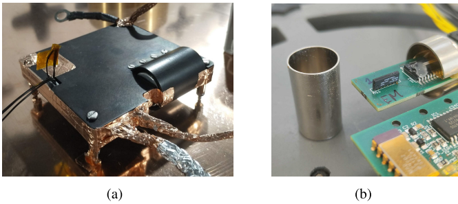
Fig. 1. (a) FM of MELISA-III during the qualification campaign and (b) one-layer magnetic shield used for the present experiment.
