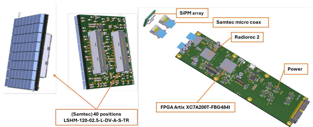
Figure 2. CAD rendering of the SiSMUV detector unit, illustrating the modular design of the SiPM array, readout electronics, and cabling adapted for spherical focal surfaces.
