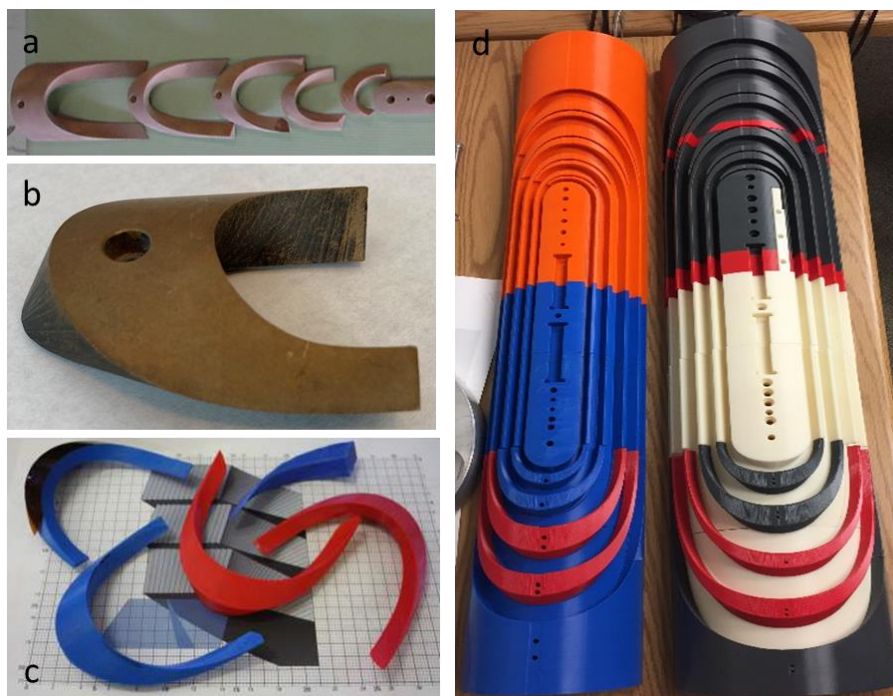
Figure 3. Practice end parts used in various cos-theta dipole coils: a) SLS end spacers; b) waterjet end spacer; c) plastic end spacers; and d) plastic parts for stress management coils.
