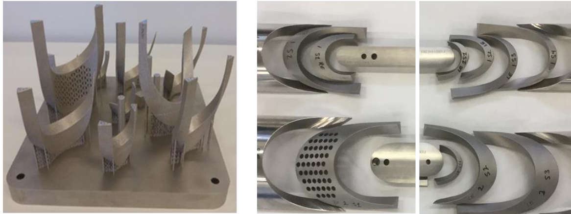
Figure 5. Spacers arrangement during printing (left) and end spacers printed on the SLM 280HL System using Ti6Al4V alloy for inner coils of the 15 T dipole demonstrator [4], [15] (right).
