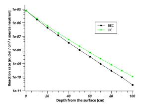
**Figure 5.** Calculated reaction rates of  $^{93}$ Nb(n,2n)  $^{82m}$ Nb reaction in BEC, OC
