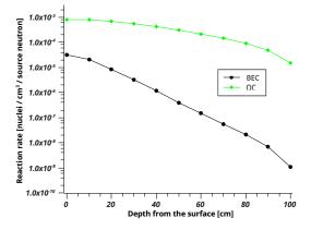
**Figure 4.** Calculated reaction rates of  $^{197}$ Au(n,  $\gamma$ )  $^{198}$ Au reaction in BEC, OC
