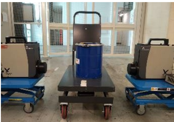
Fig. 5. View of the gamma spectrometry setup.
