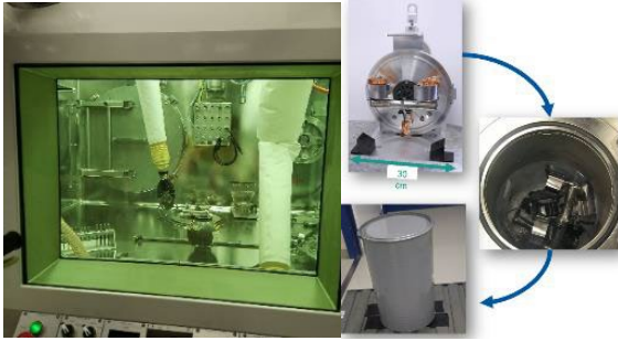
Fig. 4. (Left) view of the hot cell at the ISOLDE facility used to dismantle and package the targets into drums. (right) a process showing the packaging of the target aluminum containers into a 107 L drum.
