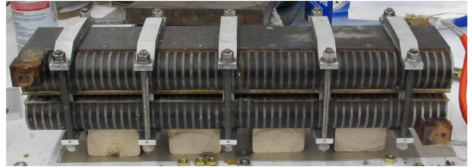
Figure 6. Second 0.5 m long Nb 3 Sn planar SCU prototype assembled at APS. © 2021 IEEE. Reprinted from [79], with necessary permissions from a contractor of the U.S. Government under Contract No. DE-AC02-06CH11357. Courtesy of ANL managed and operated by UChicago Argonne, LLC.
