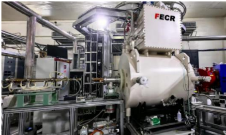
Figure 3: The world's first 45 GHz ECR ion source has been successfully developed and commissioned.
