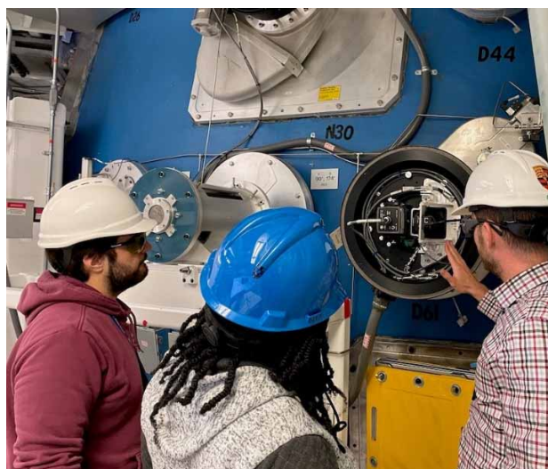
Figure 14: Cameras of the Chamber Interior Viewing System (CIVS) are mounted directly at the Target Chamber ports and subject to neutron radiation damage.
