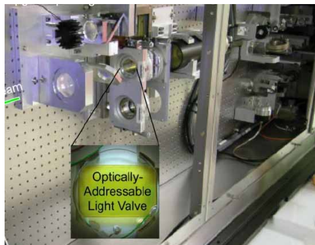
Figure 6: PSS in NIF Pre-amplifier Module (PAM).
