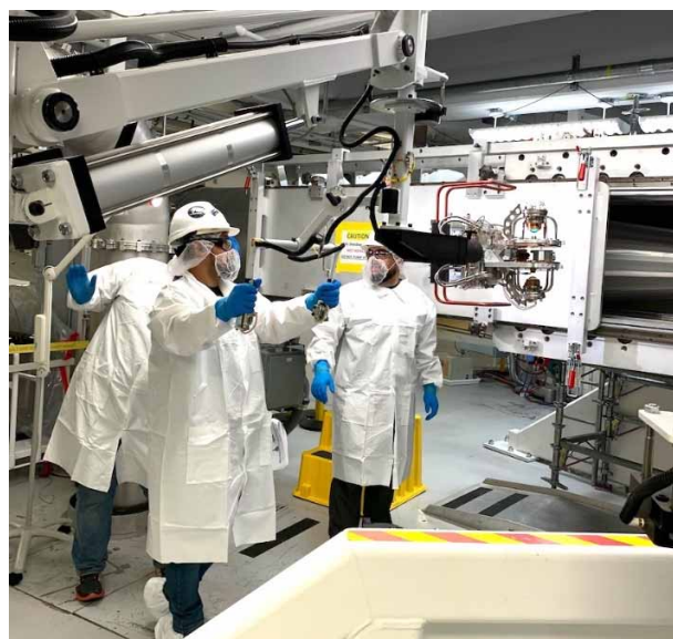
Figure 16: NIF TAS is being removed from the positioner for maintenance.
