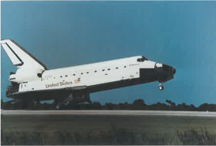
Fig. 4.3 The space shuttle Endeavor landing a Kennedy space center. The “slapdown” of the nose wheel in a worst case landing is the most severe inertial load for the design
