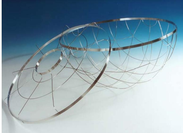
The ANTARES shield reduces the magnetic field strength on the PMT by a factor of  $\approx 3$  (and  $\approx 8$  for the NESTOR shield), with the resulting improvement in the single-
