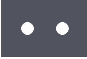
Figure 8-16: CAD rendering of the shim design for adjusting the cavity length. The shim can be placed between the cavity mirror holder and the cavity ring. Two #4 clearance holes are provided to allow through the screws used to attach the mirror holder to the cavity ring. The diameter of the clearance holes on the shim is smaller than the diameter of the clearance holes on the mirror holders. If the shims are well-positioned, then the edges of the clearance hole will not be pinched between the mirror holder and cavity ring. This is important because, as discussed in the text, the edges cut by the laser cutter are typically thicker than the rest of the shim.
