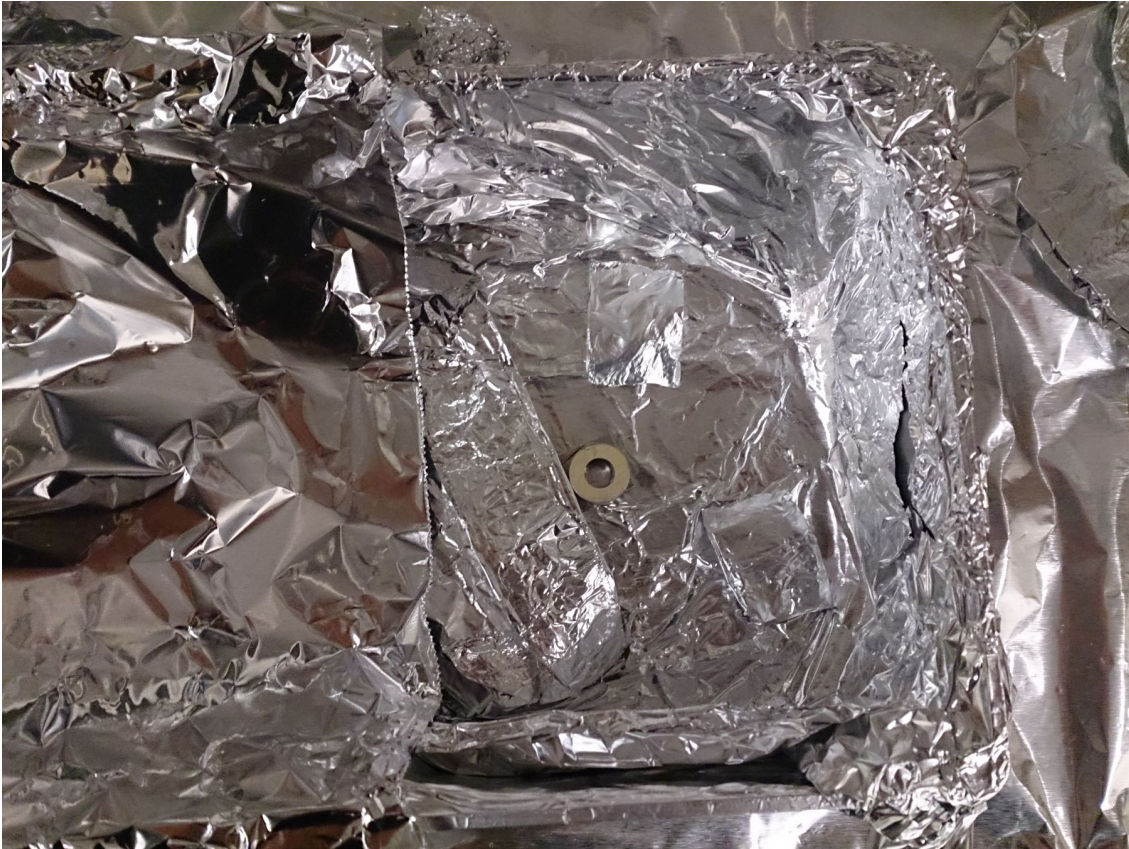
Figure 8-11: Photo of the piezo mounted inside the Faraday cage. Aluminum foil is placed over the leads to shield them. The external soldering contacts on the sides of the piezo are not shielded.
