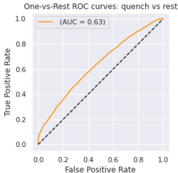
Figure 2: The ROC curve for the quench vs. rest using a MLP with PS data from BNL.
