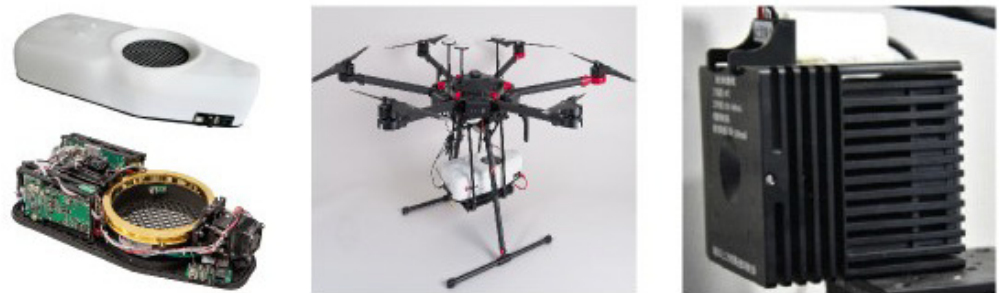
Figure 1. Airborne portable CH 4 laser spectrometer mainframe using a QCL (left), a spectrometer on-board system (middle) [32] and the wavelength of 8.9 μm and 3D dimensions of a 70 × 70 × 70 mm 3 micro QCL developed by our team (right).
