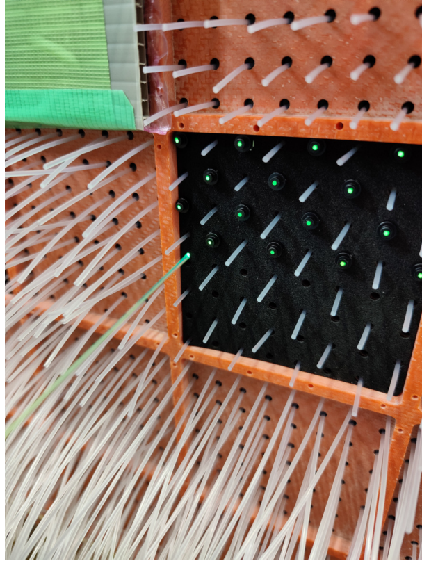
Figure 3.4: Fishing lines holding the SFGD cubes in place were removed one at a time in a checkerboard pattern when inserting wavelength shifting fibres. The MPPC connector end of the fibres are shown sitting on the foam padding.
