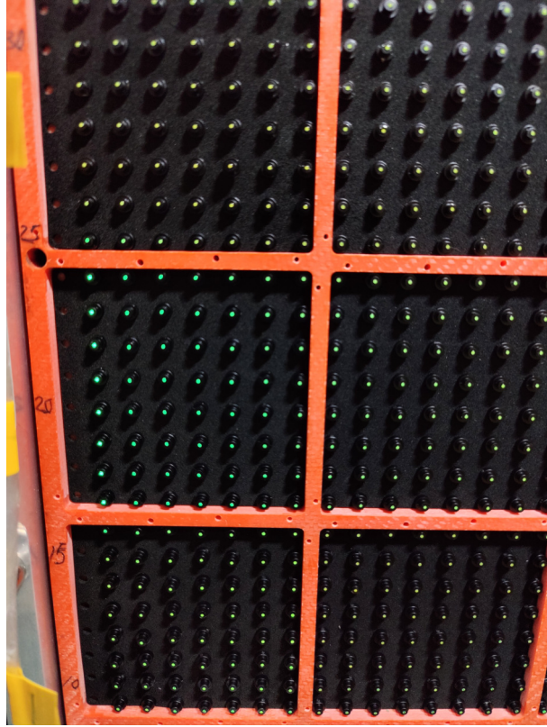
Figure 3.5: Fully installed horizontal wavelength shifting fibres on the SFGD.
