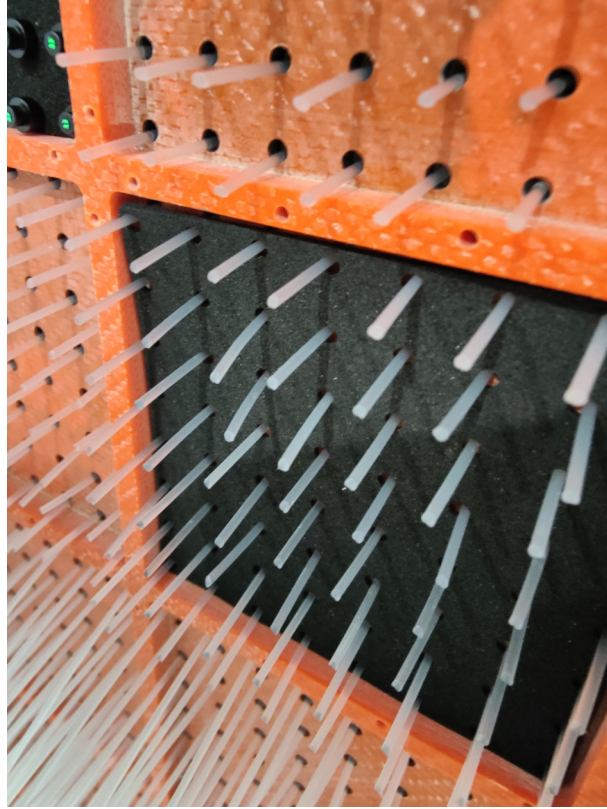
Figure 3.3: Fishing lines used to keep the SFGD cubes in place before wavelength shifting fibres were installed. A custom foam square was placed over all 64 fishing lines. This foam provided padding for the MPPC connector at the end of the wavelength shifting fibre.
