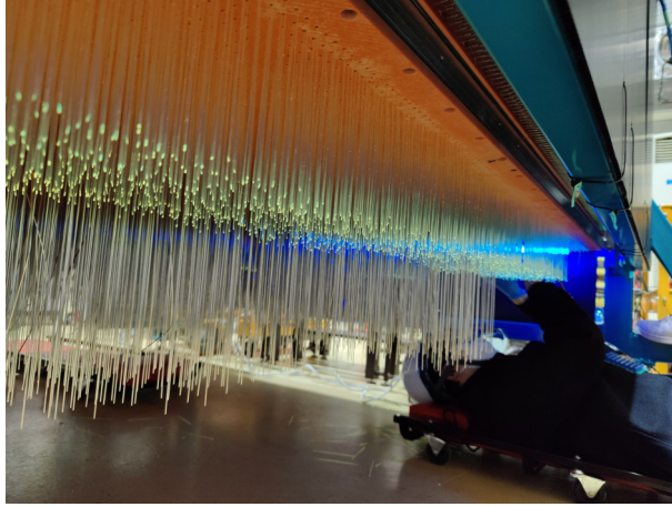
Figure 3.7: Vertical wavelength shifting fibres leaving the SFGD box. These fibres were cut to a length of 5 cm for a quality control test. This tested if any fibres were damaged during insertion. The right side of the image shows this test being performed with a blue LED array.
