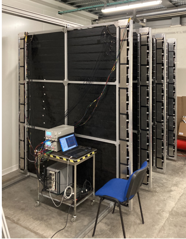
Figure 2.24: The TOF planes at CERN for testing with cosmic rays. Figure from Ref. [90].
