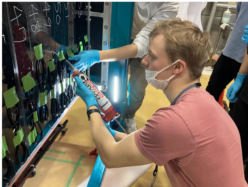
Figure 3.17: A picture of the author applying the caulk glue to the gaps between the SFGD modules.
