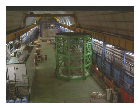
Figure 4.3: The external dewar of the 100 l WArP detector surrounded by the shielding structure on site in the underground laboratory at Gran Sasso.
