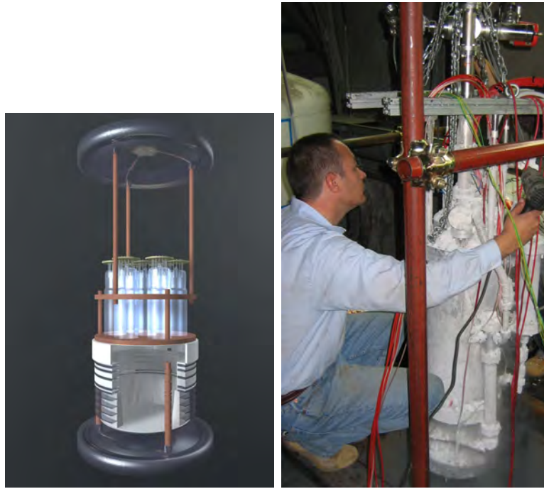
Figure 4.6: The WArP 2.3 liter detector layout and a picture of the chamber being dismantled.
