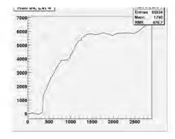
Figure 4.8: The primary signal from the WArP detector. a) A raw form, b) an integrated waveform.
