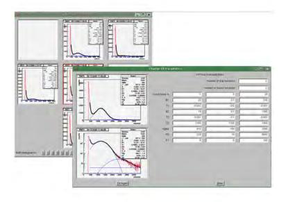
Figure 5.2: The SER fitting program used for the ongoing calibration of the WArP chamber. The main window is shown as well as the auxiliary window used to fit single PMTs if the fit with the standard parameters did not converge.
