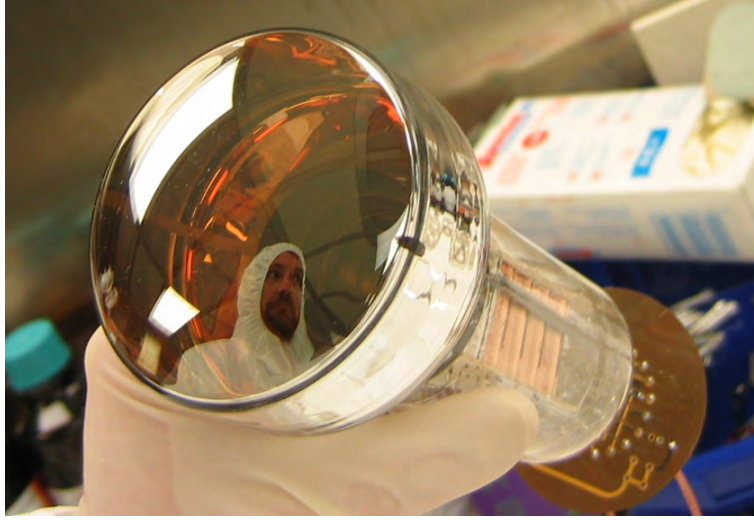
Figure 4.5: One of the 3" photomultipliers used in the WArP 2.3 liter prototype. The multiplying dynodes are visible on the right, as well as the light collecting window.
