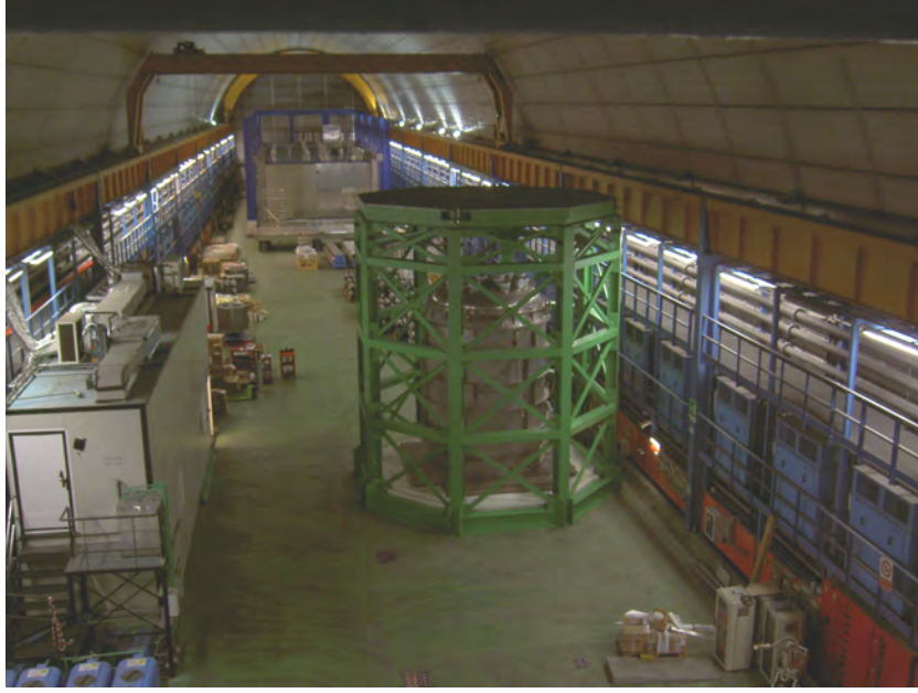
Figure 4.3: The external dewar of the 100 l WArP detector surrounded by the shielding structure on site in the underground laboratory at Gran Sasso.
