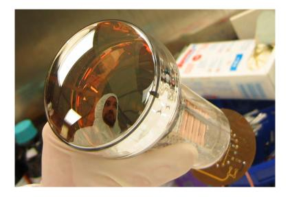
Figure 4.5: One of the 3" photomultipliers used in the WArP 2.3 liter prototype. The multiplying dynodes are visible on the right, as well as the light collecting window.
