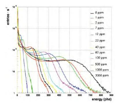
Figure 5.10: <sup>60</sup>Co spectra measured with different quantities of gaseous nitrogen injected into the test chamber. Only the Compton edge is visible in most cases, the full absorption peak is not very pronounced [106].
