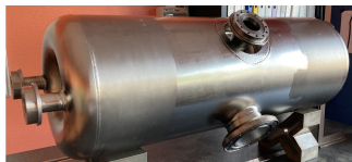
Figure 8: Picture of the naked high beta cavity before cryogenics tests.
