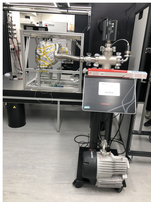
(b) Chamber wrapped in foil (used to bake the chamber) and the vacuum pump during vacuum pumping
