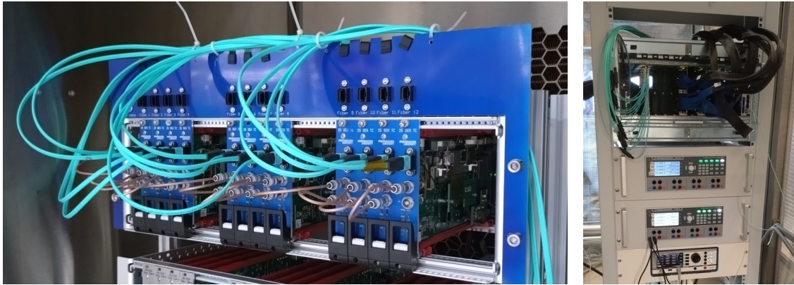
Figure 8.1: Crate-based Service Hybrid test setup at CERN. Left: fully installed crate with 2S-SEH test cards inside the climatic chamber. Right: rack adjacent to the climatic chamber with auxiliary devices.
