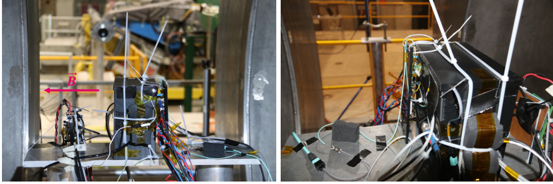
Figure 6.3: Left: the three tested Outer Tracker devices after installation on the table inside the M1 magnet. From left to right: a PS-POH, a 2S module in a light-tight box, and a SEH. They are all in endcap configuration. Right: close-up of the SEH installation in endcap configuration.
