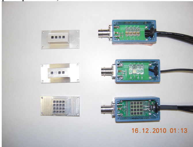
Fig. 3. From the top, on right: 4 STM inside the Pomona box with printed circuit board. The support for radiators or crystals is on the left. The same for 1 STM is in the middle. The MPPC matrix, 4x4 cells inside Pomona box with printed circuit board and support for radiators or crystals are on the bottom.
