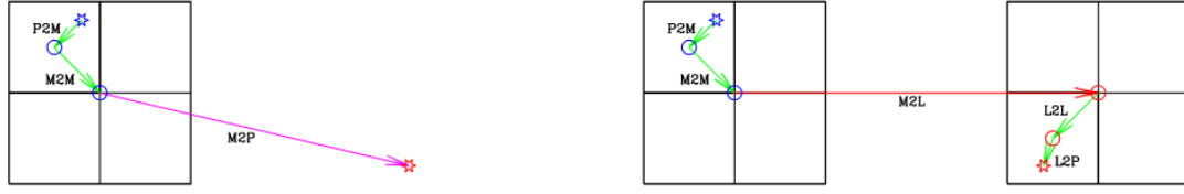
Figure 2.3: Comparison of tree code (left) and FMM (right) algorithms. From Dehnen (2014) .
